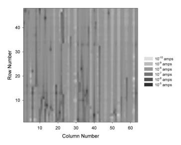
Figure 14. Reverse bias current/pixel for a  $48 \times 64$  display with  $V_{reverse} = 6V$
