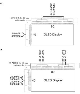
Figure 4. Connection schematic for two Model 7015-C scanner cards and a 40×80 sample display with a) two Model 2400 SourceMeter instruments b) four Model 2400 SourceMeter instruments.
