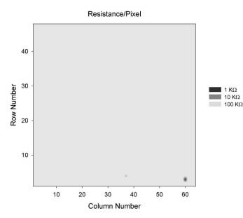
Figure 11. Resistance/pixel with an applied bias of  $V_{bias} = 2V$
