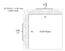
Figure 3. Connection schematic with two 7015-C scanner cards and a 40×40 sample display with a 2400 SourceMeter instrument.
