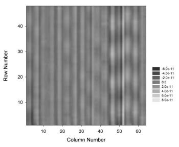
Figure 13. Residual test system leakage current/pixel with an applied bias of  $V_{bias} = -6V$
