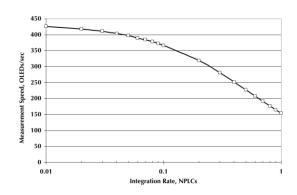
Figure 10. Measurement throughput of the OLED characterization system with four Model 2400s
