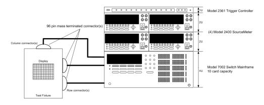
Figure 5. Diagram of the OLED characterization system with Model 7002 Scanner Mainframe, Model 2361 Trigger Controller and four Model 2400 SourceMeter instruments.
