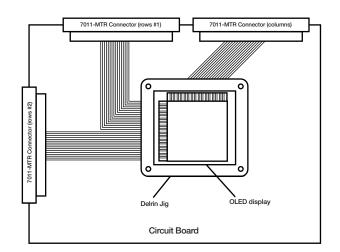
Figure 6. Top view of an OLED test fixture for a 48×64 display
