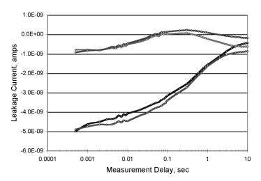
Figure 8. Reverse bias current/pixel for four pixels with a source/measure delay from 0.0005 to 10 seconds with an applied bias of 6V
