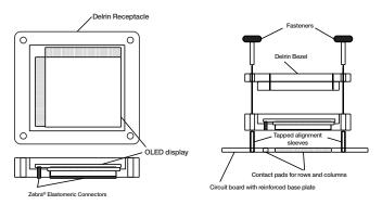
Figure 7. Detail views of the jig designed for a 48×64 OLED display
