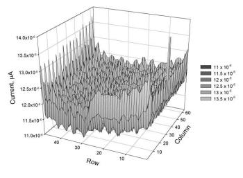
Figure 12. Current consumption/pixel with an applied bias of  $V_{bias} = 6V$
