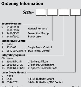
Select the instrument and accesory for your application. Review the detailed specifications of each instrument in individual catalog sections.
