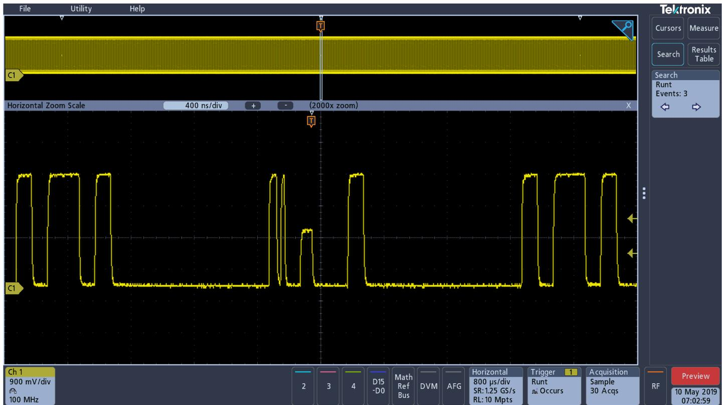
FastAcq helps with revealing the presence of runt pulses in the digital data stream for further investigation. In this test case, Search revealed and marked 3 runt pulses in the 10 Mpoints acquisition.
