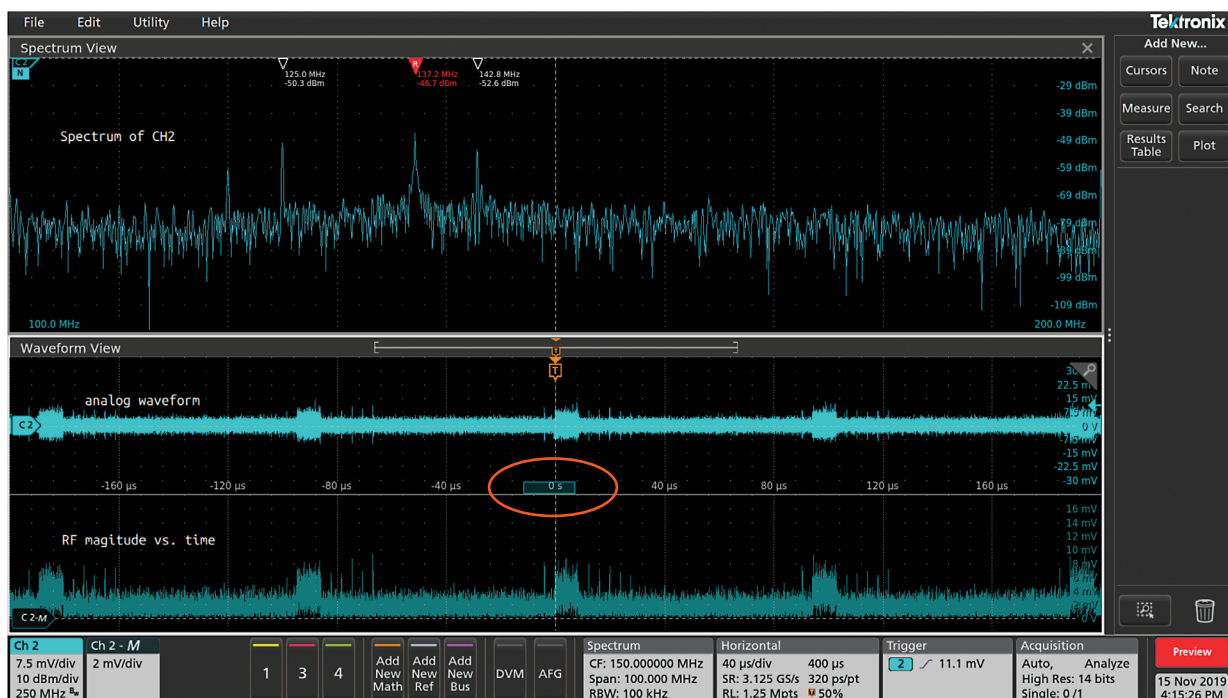
FIGURE 13. The center trace is the time-domain waveform from the H-field probe. The spectrum content corresponding to the spectrum time indicated by the blue block below the waveform (circled in orange). The RF Amplitude vs. Time trace (bottom) shows a repetitive RF burst.
