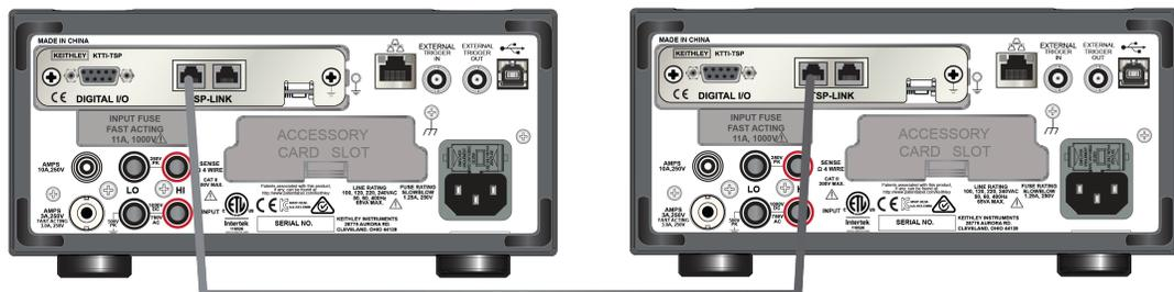
3. Connect the computer to the DMM6500 that is set to node one.
