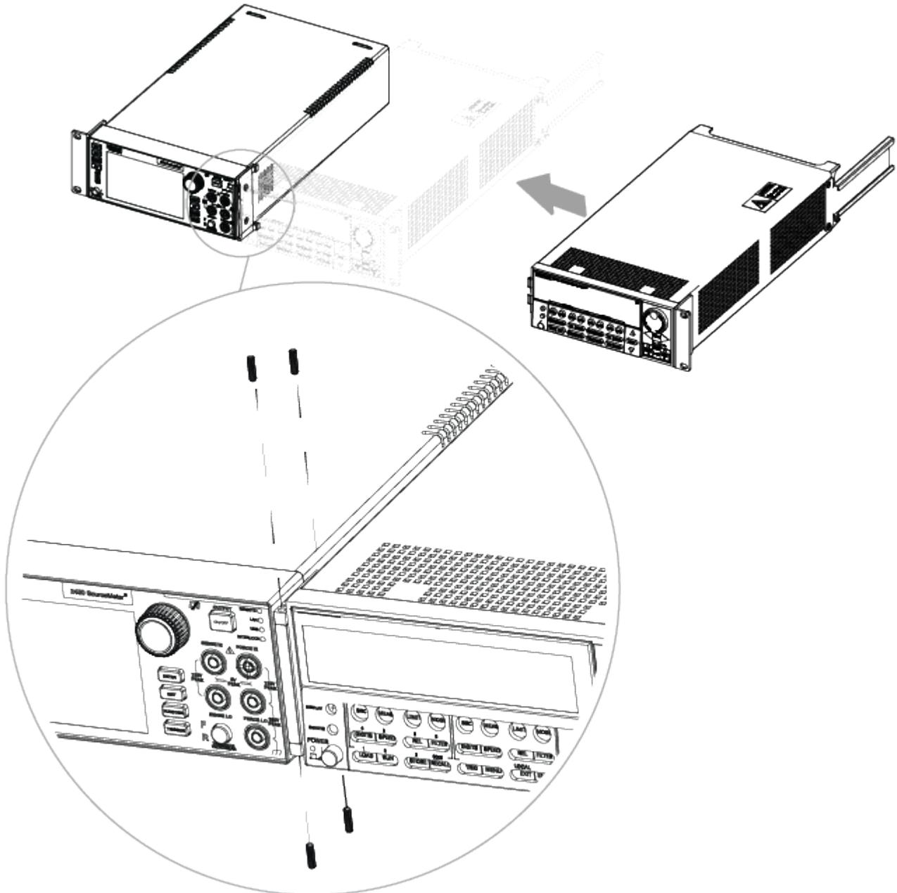
**To install the mounting hardware on the instruments:**
