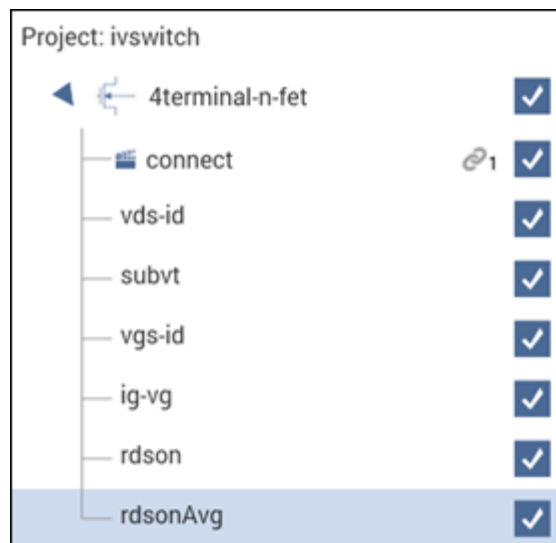
Figure 34: Project tree with rdsonAvg added to 4terminal-n-fet device
