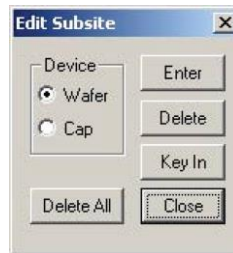
Figure 317: CM500 Prober Edit Subsite window
