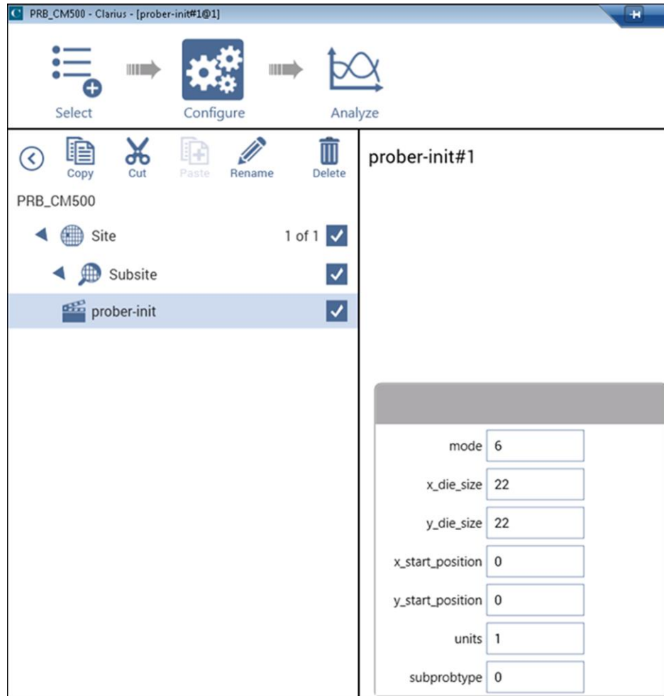
Figure 321: Set prober-init parameters
