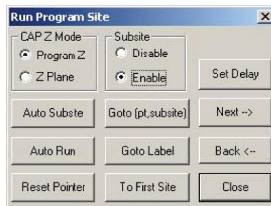
Figure 318: CM500 Prober Enable Subsite
