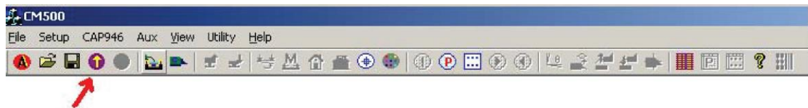
Figure 298: CM500 Prober load wafer icon
