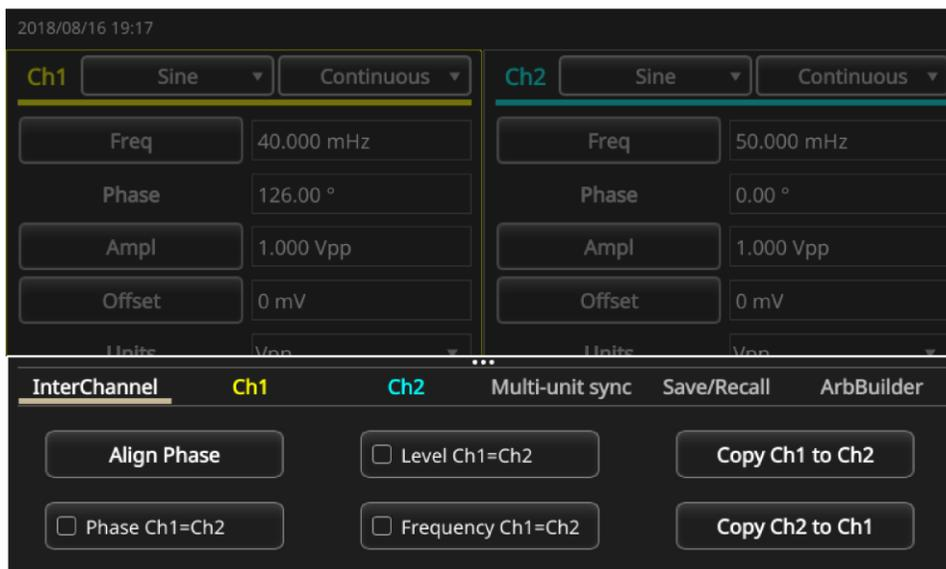
Figure 47: Copy channel 1 to channel 2
