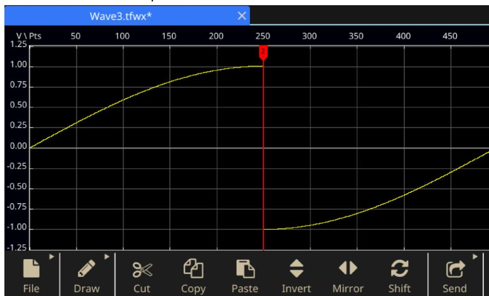
Figure 132: ArbBuilder highlight waveform data to cut
