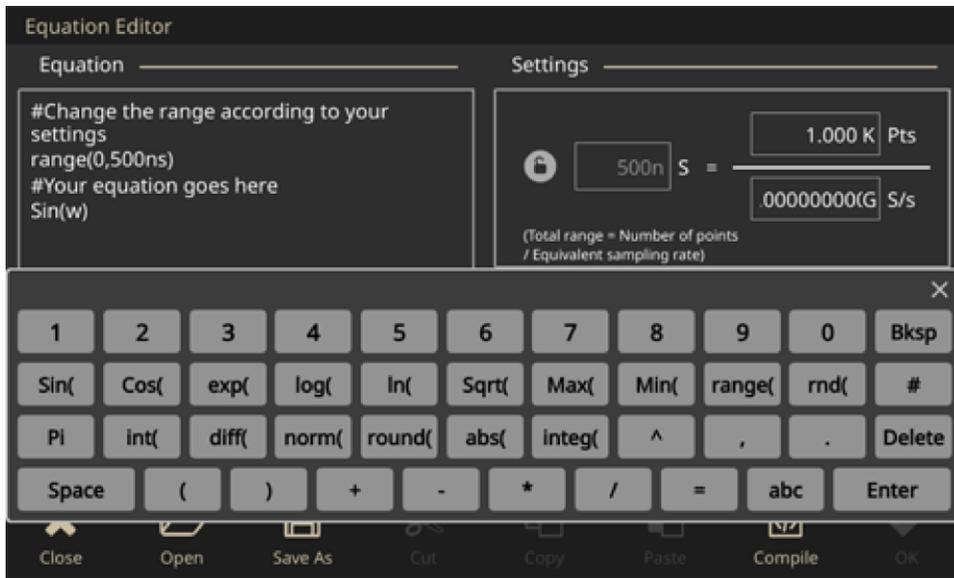
Figure 120: ArbBuilder equation file with soft keyboard
