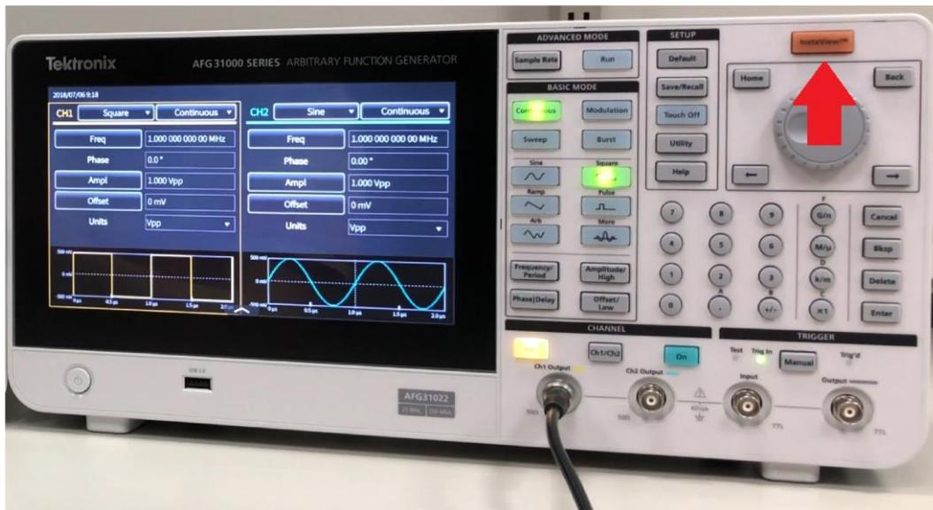
**Figure 67: Set up InstaView on the AFG31000 instrument**
