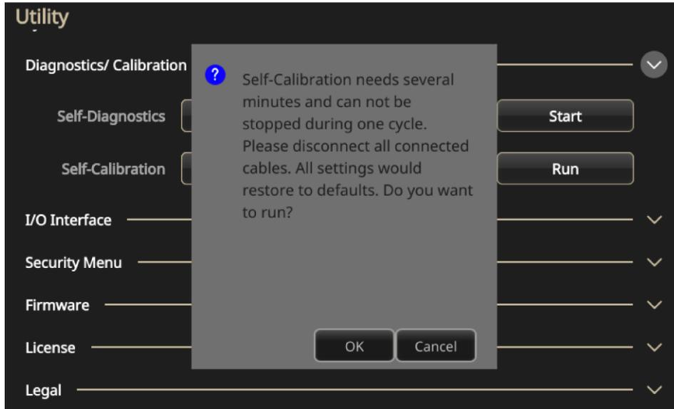
**Figure 110: Run self-calibration**
