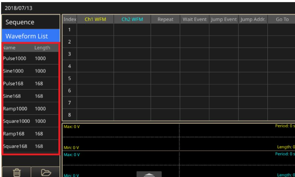
Figure 93: Select from the Waveform List
