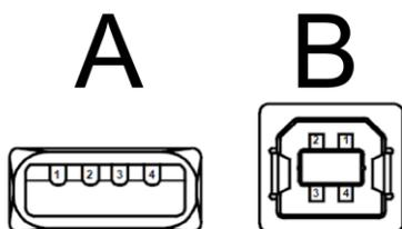
Figure 16: Type A and B USB connectors
