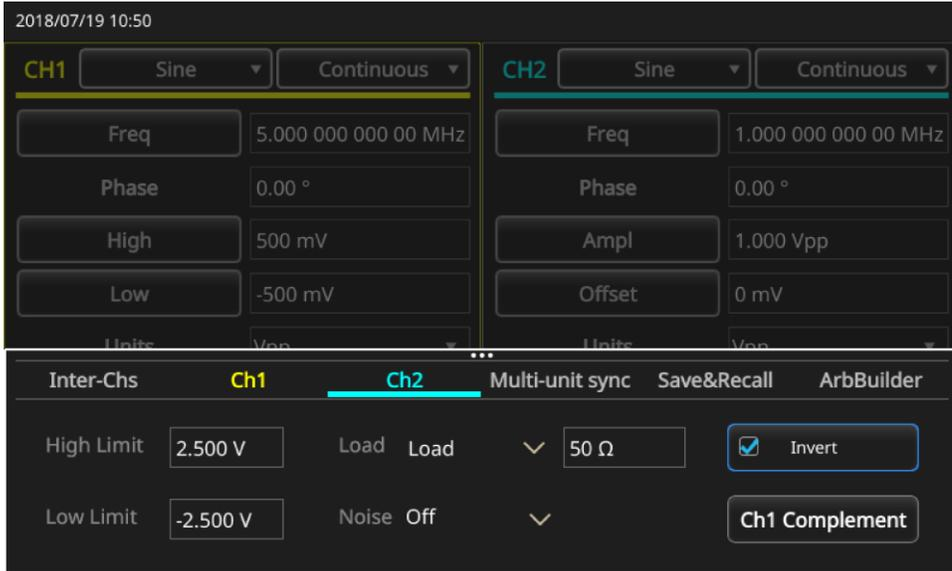
**Figure 48: Invert channel 1 and channel 2 wave polarity**
