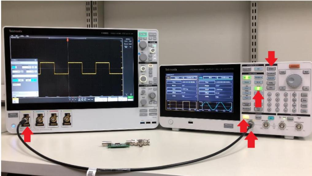
Figure 65: AFG31000 InstaView setup with connections overview
