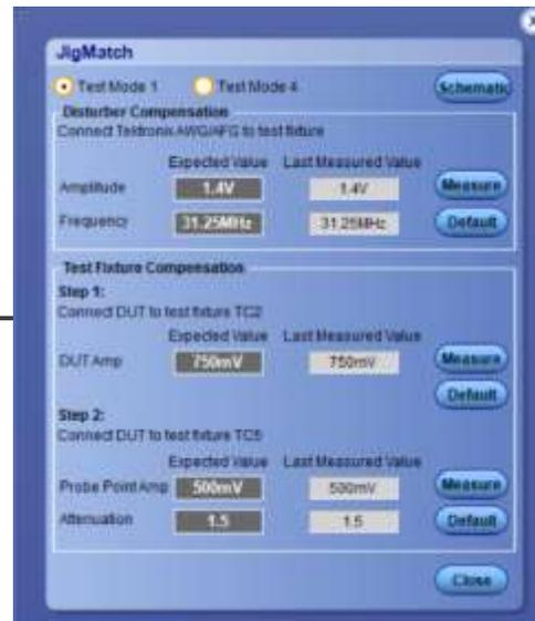
JigMatch calibrates the Disturber source as per the specification
