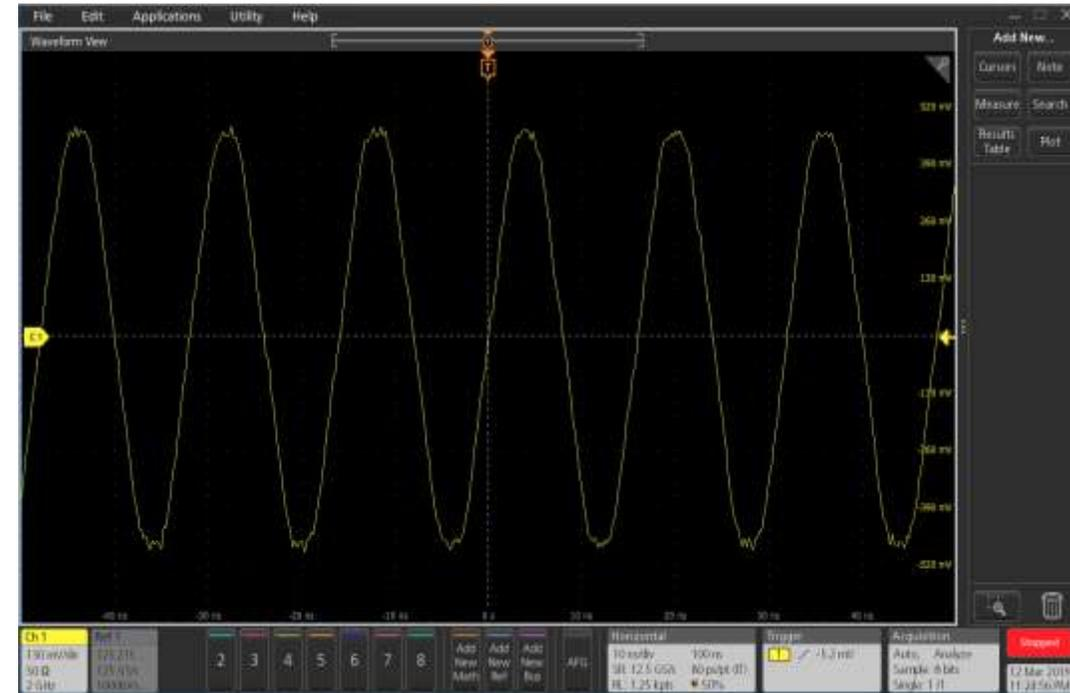
*1000BASE-T Test Mode-2 waveform*
