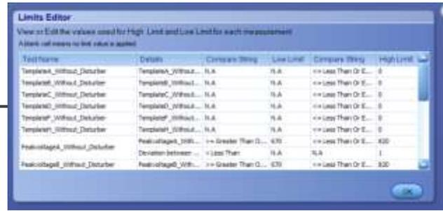
Limits editor enables you to define the limits beyond compliance requirement and test the DUT for design margins
