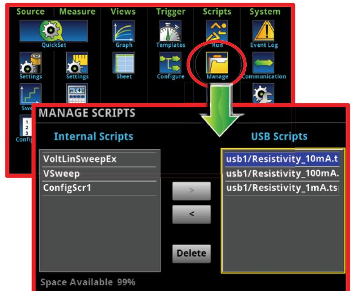
**Figure 6.** The Manage Scripts window enables the user to download scripts from a USB drive and store them into non-volatile memory.
