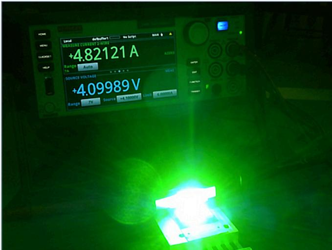
**Figure 6.** HBLE LED illuminated at 4.1 volts and 4.8 amps
