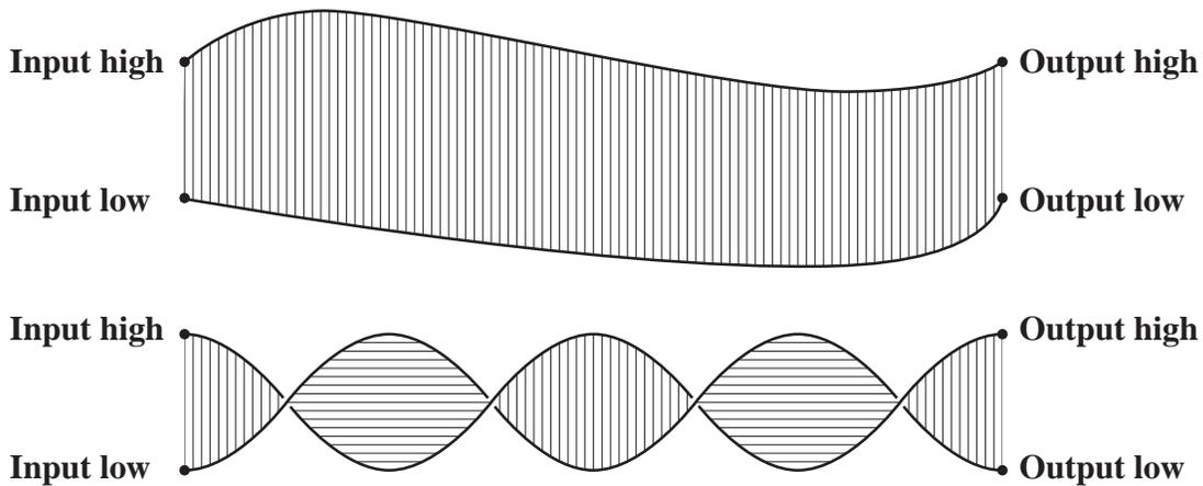
Figure 1. Magnetically induced noise voltages are proportional to the area of the current loop formed by the signal leads (top). Twisting the leads can virtually eliminate those voltages. Noise contributions from the horizontally shaded loop areas cancel contributions from those with vertical shading.
