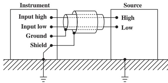
from surrounding the actual signal lines with a guard electrode tied to signal low, and surrounding that with a shield tied to ground.
