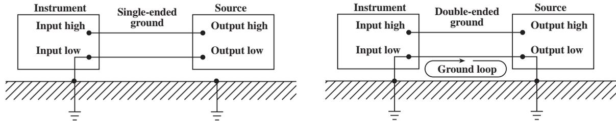
second point creates a ground loop that soaks up any available AC magnetic field energy and applies it directly to the measurement input.
