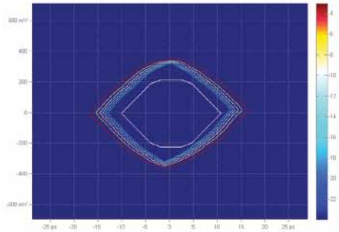
Figure 5a. Eye mask testing with BER contours. The  $BER=10^{-6}$  contour, the outer yellow-orange contour, corresponds to a  $5 \times 10^{-5}$  hit ratio.
