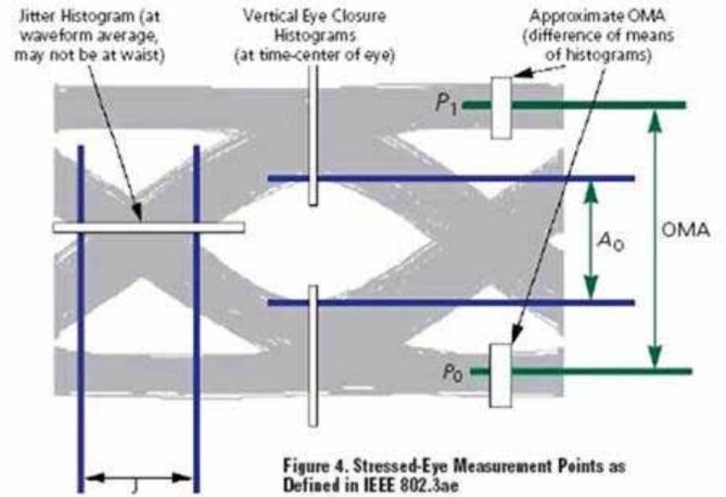
Figure 4. Stressed-Eye Measurement Points as Defined in IEEE 802.3ae
