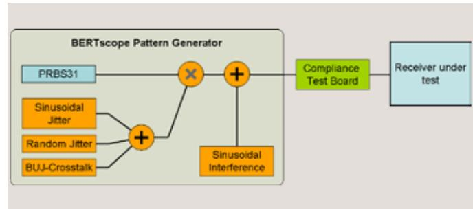
**Figure 14.** Electrical stressed receiver test setup.
