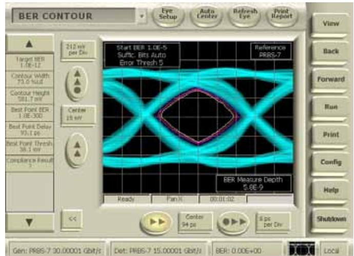
Figure 5b. BER Contour for J9 with BERTScope using a 30 Gb/sec signal.
