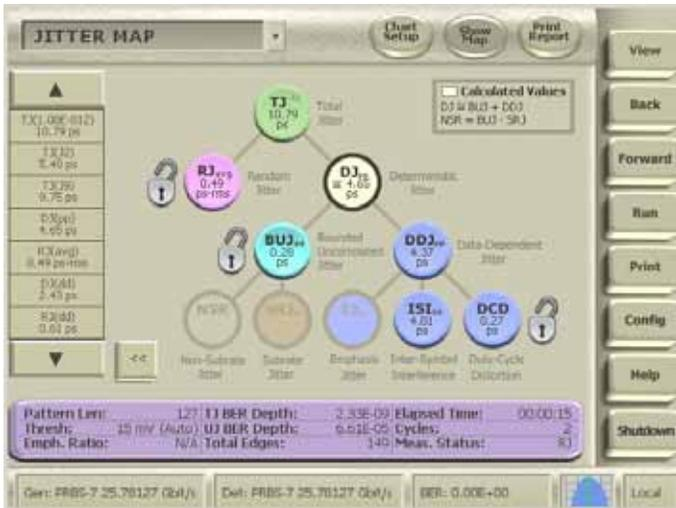
Figure 16. Example of jitter decomposition on a BERTScope.
