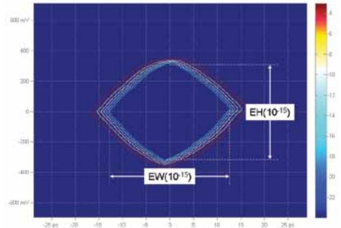
Figure 13. Measurements of EH(10<sup>-15</sup>) and EW(10<sup>-15</sup>) with a BER Eye diagram.
