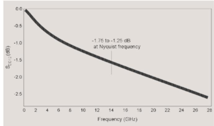
Figure 12. Differential frequency response of typical compliance test boards.
