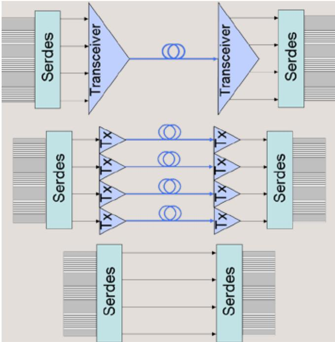
**Figure 2.** Diagram of (a) 4x25 Gb/s 100G Serdes-Transceiver WDM optical system, (b) 4x25 Gb/s 100G Serdes-Transceiver optical system, and (c) a 4x25 Gb/s 100G Serdes to Serdes electrical system. The figure does not show the symmetric return paths.
