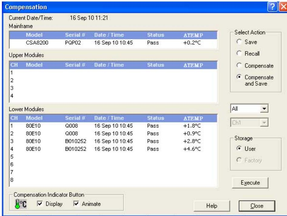
Figure 1 Compensation pane of the DSA8200 Oscilloscope.
