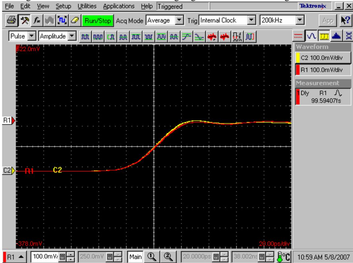
**Figure 18 Delay measurements between the reference (R1) acquired from the channel one and the channel two (C2). It has to be the minimum for the best deskew value.**
