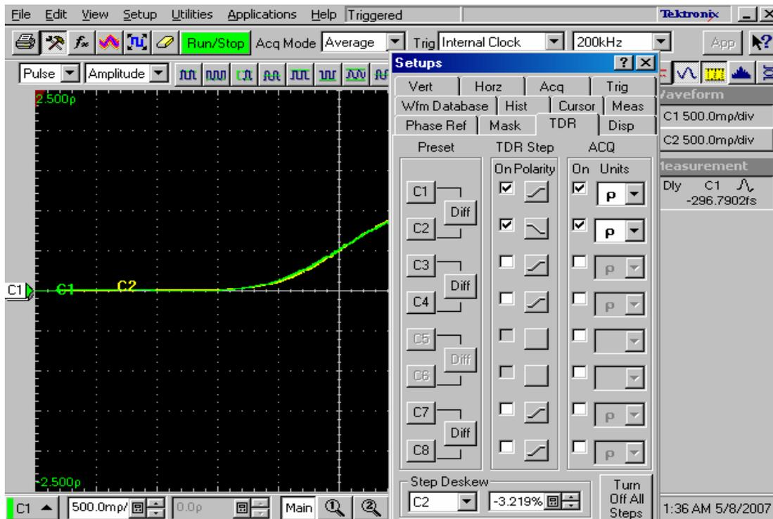
Figure 19 Differential TDR step deskew. The channels C1 and C2 are aligned within ~300fs.
