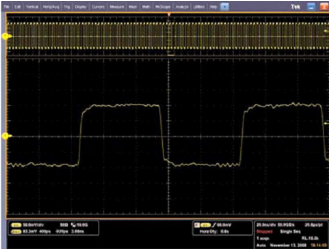
Figure 16a. Oversampled waveform using \sin(x)/x interpolation.
