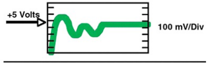
Figure 8: Vertical offset changes the volts/div reference point from zero, to some other voltage.
