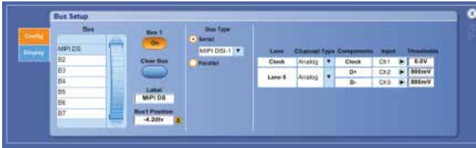
Figure 51. MIPI DSI-1 Bus Setup.
