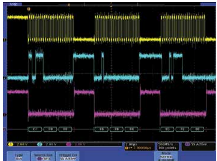
Figure 12. Acquiring synthesizer configuration messages off the SPI bus.
