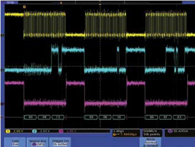
Figure 13. Correct synthesizer configuration messages.
