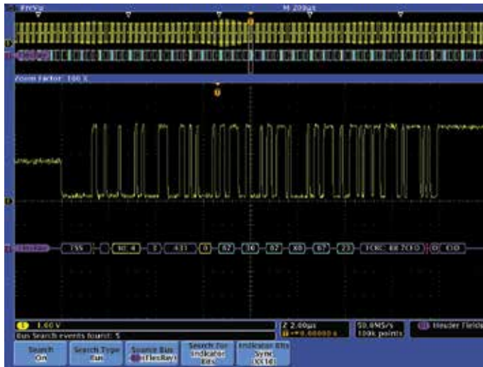
Figure 42. Triggering on Frame ID and Cycle Count, Searching through acquired data for Startup Frames.
