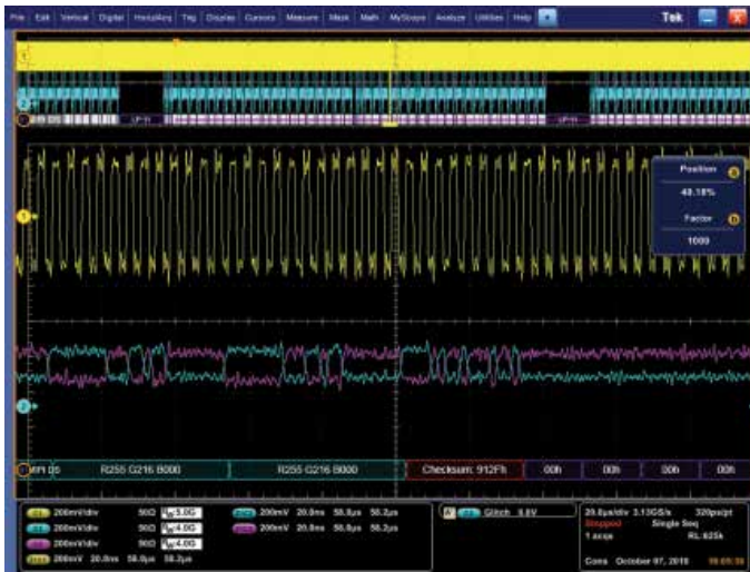
Figure 53. MSO70000C analog-channel decoded display of a Packed Pixel Stream, showing a checksum error.
