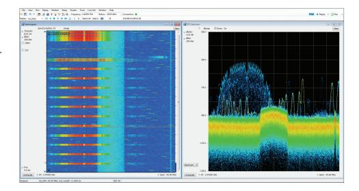
operating on 2.437 GHz (Wi-Fi Channel 6). There are also more than 10 other signals in the display at varying frequencies and power levels. Given the spectrum shape and frequencies in use, these signals are probably from a Bluetooth device. >>
