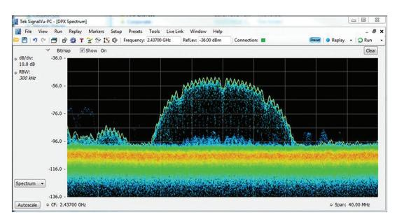
One of the key differences between an RTSA and a basic signal analyzer is in the RTSA bandwidth specification. For any span up to the maximum real-time span, an RTSA does not have to sweep and is able to continuously capture spectrum information. An RTSA is also not limited to a single display at one time. Spectrum, spectrogram and modulation information can be simultaneously analyzed and because this data is from a continuous acquisition, the information is timecorrelated.
