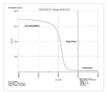
Figure 3. C-V curve of a p-type MOS capacitor measured with the  $\ensuremath{\texttt{4210-CVU}}$
