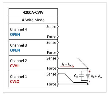
Figure 7. Configuration for C-V characterization of a diode using the  $\ensuremath{\texttt{4200A-CVIV}}$
