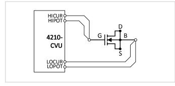
Figure 14. C-V test configuration for a MOSFET.
