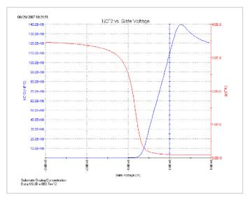
Figure 6. 1/C<sup>2</sup> vs. gate voltage plot generated with 4210-CVU
