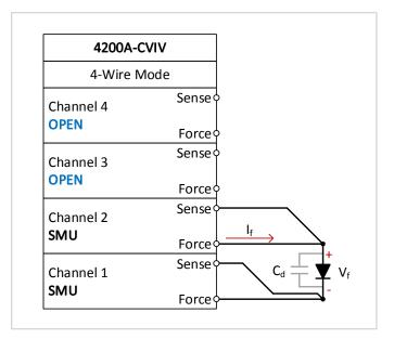
Figure 6. Configuration for I-V characterization of a diode using the  $\ensuremath{\texttt{4200A-CVIV}}$
