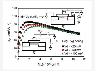
Figure 2. Effective channel mobility measured by conventional technique.  $I_{ch}$  was measured under various non-zero drain biases,  $V_{\rm DS^{\prime}}$  but  $Q_i$  was measured under  $V_d=0$ . The extracted mobility clearly reduces for higher  $|V_d|$ . Insets illustrate the carrier distribution in the channel.
