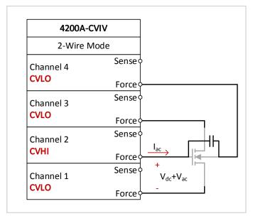
Figure 15. C-V characterization of a four-terminal MOSFET using the  $\ensuremath{\texttt{4200A-CVIV}}$
