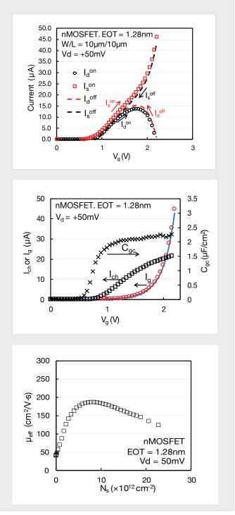
Figure 8. (a) Four currents measured from the source and drain corresponding to the off-to-on and on-to-off V<sub>g</sub> sweeps by UFSP technique on an nMOSFET with EOT of 1.28nm.
