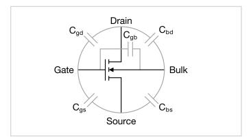
Figure 13. Parasitic capacitances of a MOSFET.
