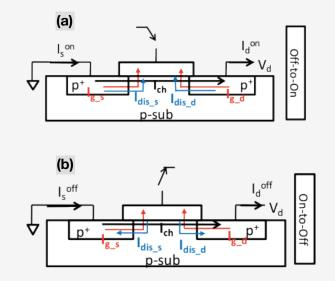
Figure 4. Schematic diagram of current flow during the transient measurement.
