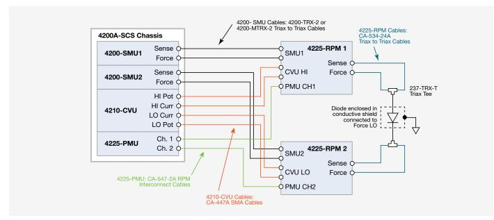
Figure 4. Connections from the 4200A-SCS and 4225-RPMs to the diode.
