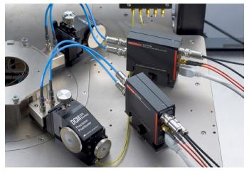
Figure 2. The output terminals of each 4225-RPM module connect to a single prober.
