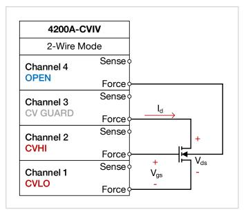
Figure 12. I-V characterization of a four-terminal MOSFET using the  $\ensuremath{\texttt{4200A-CVIV}}$
