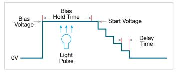
Figure 11. Preferred C-V measurement Sequence The device is first biased at the "PreSoak" voltage for the
