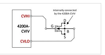
Figure 16. 4200A-CVIV two-terminal MOSFET C-V test equivalent circuit.
