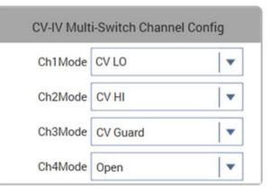
Figure 10. *cviv-configure* settings for a base-emitter capacitance measurement on a BJT.
