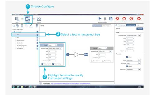
Figure 7. Configure tests in the diode project.
