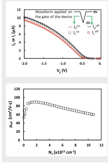
Figure 6. (a) I<sub>ch</sub>, I<sub>g</sub>, and C<sub>gc</sub> extracted simultaneously from the currents in Figure 5 by using Equations (2)–(5). (b) Channel effective mobility extracted from I<sub>ch</sub> and C<sub>gc</sub> from (a).
