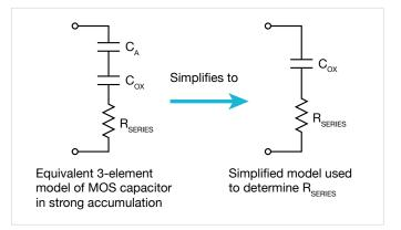
Figure 12. Simplified model to determine series resistance
