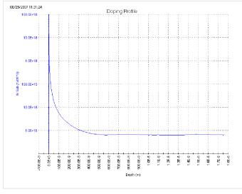
Figure 7. Doping profile extracted from C-V data taken with 4210-CVU
