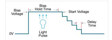
Figure 11. Preferred C-V measurement Sequence
