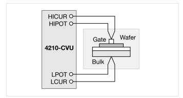
Figure 8. Basic configuration to test MOS capacitor with 4210-CVU
