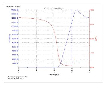
Figure 6. 1/C<sup>2</sup> vs. gate voltage plot generated with 4210-CVU
