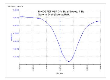
Figure 6. VLF C-V Sweep of an n-MOSFET measured between the gate to drain/source/bulk. This graph is from the vlf\_nmosfet\_vsweep\_dual test (user module vlfcv\_measure\_dual\_sweep\_bias\_fixed\_range).
