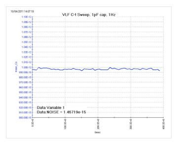
Figure 9. Results of C-t measurements of nominal 1pF reference capacitor, using VLF capacitance technique at a test frequency of 1Hz. This graph is from the *vlf-cap-time* test (user module *vlfcv\_measure\_sweep\_time*).
