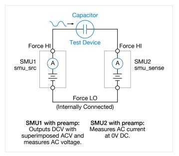
Figure 1. Connections for very low frequency C-V measurements.
