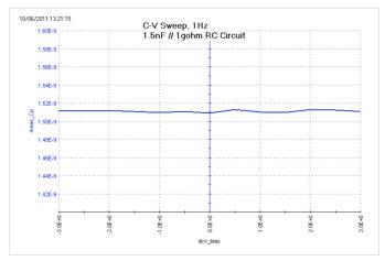
Figure 14. Results of measuring parallel RC combination of 1.5nF capacitor and  $1G\Omega$  resistor. This graph is from the vlf-1nF-1gohm test 1nF-1gohm test 1nF-1gohm
