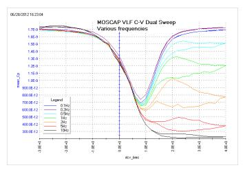
Figure 11. A VLF C-V sweep of a MOScap at various frequences from 100mHz to 10Hz created using the MOS Capacitor VLF-CV Project. This graph is from the vlf-moscap-vsweep-dual test (vlfcv\_measure\_sweep\_bias\_fixed\_range\_user\_module).
