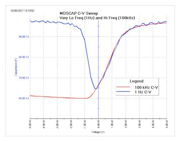
Figure 12. This graph is from the *moscap-vsweep-hif-lof* test, showing the high frequency data from the 4210-CVU card along with the VLF C-V data from the *vlf-moscap-vsweep* test.
