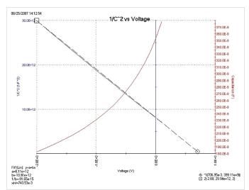
Figure 13. 1/C<sup>2</sup> vs. voltage of a silicon solar cell
