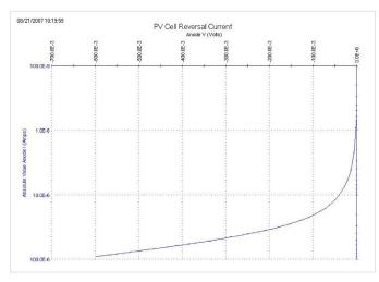
Figure 10. Reverse-biased I-V measurement of silicon solar cell using the 4200-SMU
