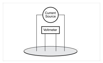
Figure 18. Four-point collinear probe resistivity configuration
