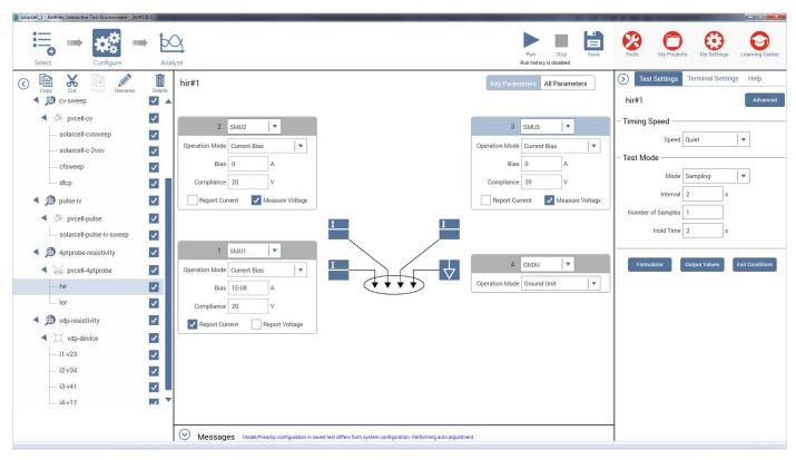
Figure 19. "hir" test module for measuring resistivity
