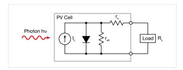
Figure 2. Idealized equivalent circuit of a photovoltaic cell
