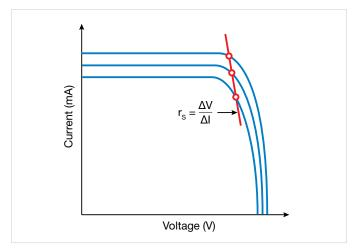
Figure 8. Slope method used to calculate the series resistance
