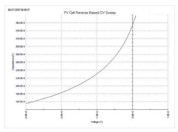
Figure 12. C-V sweep of a silicon solar cell
