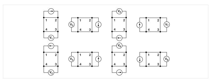
Figure 22. van der Pauw resistivity measurement conventions
