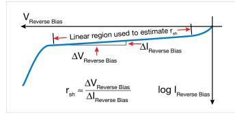
Figure 9. Typical reverse-biased characteristics of a PV cell
