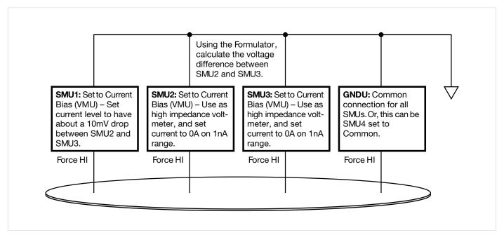
Figure 20. SMU designation for four-point collinear probe measurements
