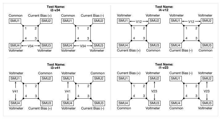
Figure 25. SMU configurations for van der Pauw measurements
