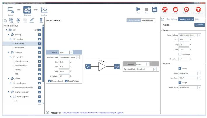
Figure 1. Screenshot of Solar Cell project for the 4200A-SCS
