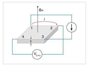
Figure 27. Hall voltage measurement
