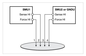
Figure 21. Connecting two SMUs for four-point probe measurements
