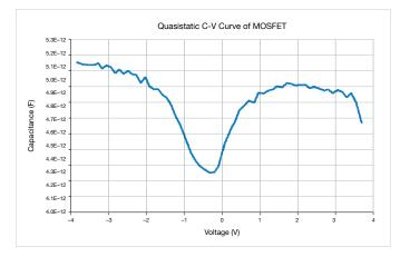
Figure 4. Quasistatic C-V Sweep of MOSFET device
