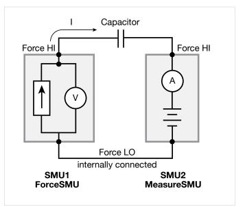
Figure 1. Connections for Capacitance Measurements Using Ramp Rate Method
