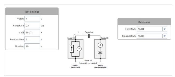
Figure 3. Configuration pane for ramprate-cvsweep test
