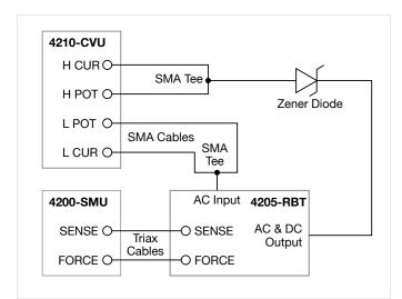
Figure 4. High Voltage C-V Connections for Zener Diode
