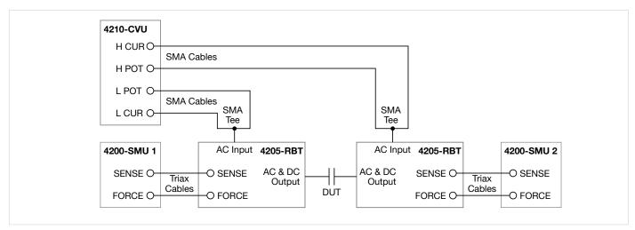
Figure 2. High Voltage C-V Measurements Using Two Remote Bias Tees
