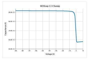
Figure 7. High Voltage C-V Sweep of MOScap
