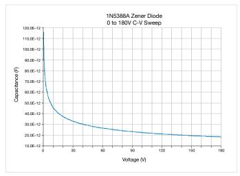
Figure 5. Results of C-V Sweep of Zener Diode
