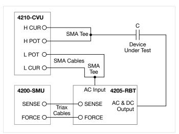
Figure 1. Device Connections for High Voltage C-V Measurements Using One Bias Tee
