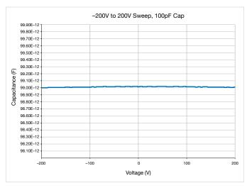
Figure 9. ±200 C-V Sweep on 100pF Capacitor
