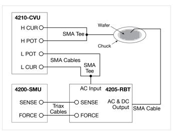
Figure 6. High Voltage C-V Connections for MOScap Testing
