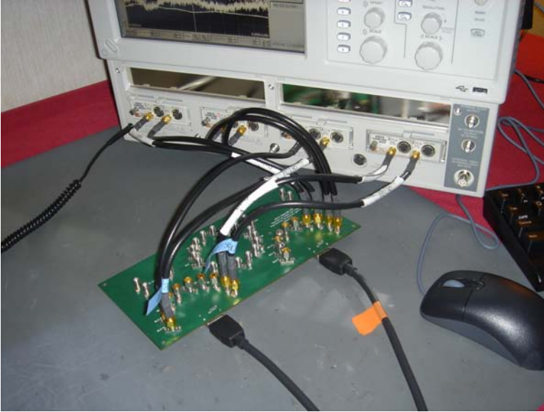
Figure 1 DisplayPort passive cable test setup.
