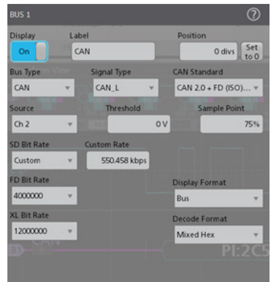
Figure 8. Configuration menu for Mixed mode CAN.
