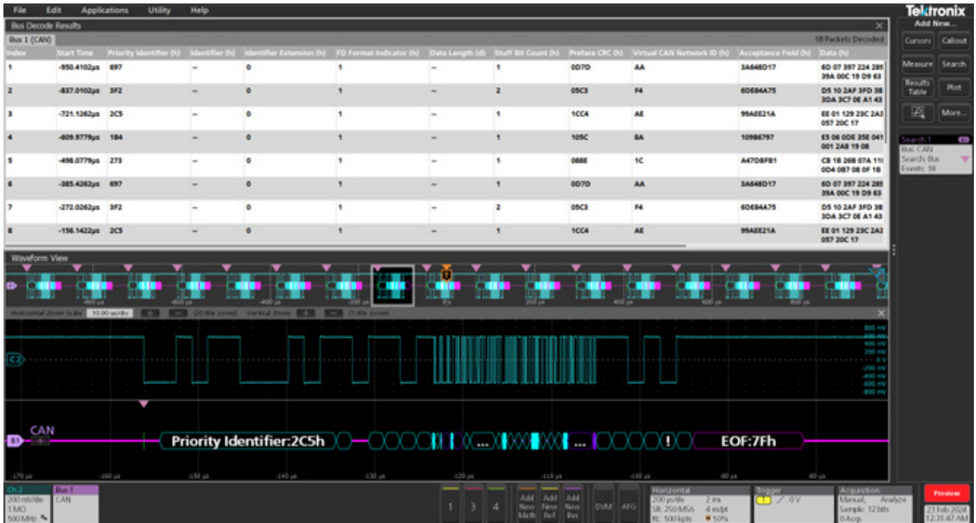
Figure 1. Decode of a CAN XL Data Frame packet.
