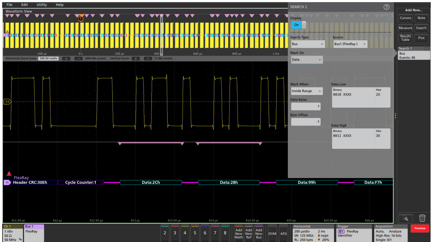
Figure 18. Wave inspector search configured to mark data inside the range 2X hex and 3X hex.
