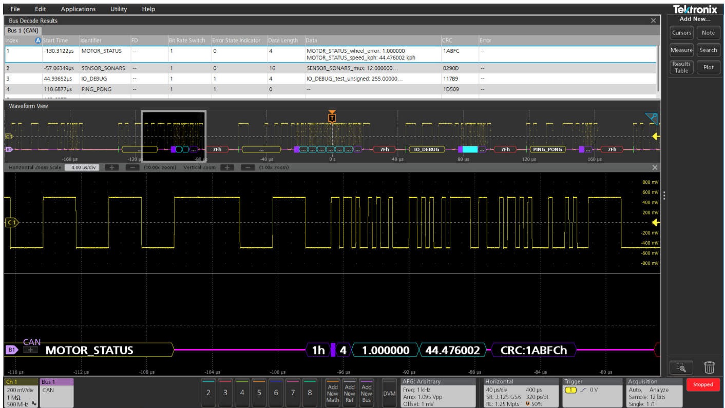
Figure 4. Symbolic message and signal values shown in the bus waveform and results table displays.
